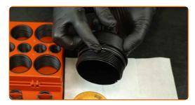
Install a new filter element into the oil filter cap.
