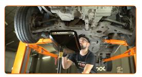
Clean the area of the oil pan drain hole. Use a wire brush. Use an all-purpose cleaning spray.
