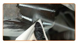
Screw in the drain plug and tighten it. Use a 13 mm socket. Use a torque wrench. Tightening torque: 23 N·m.
