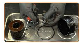
Clean the oil filter cap. Use an all-purpose cleaning spray.
