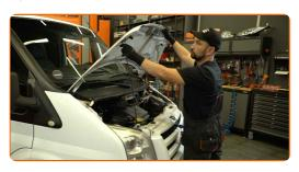
Use a fender protection cover to avoid damaging the paintwork and plastic parts of the car.
