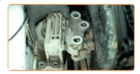
Clean the mounting seats of the engine mount. Use a wire brush. Use an all-purpose cleaning spray.
