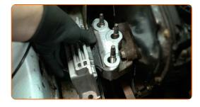
11 Install the fastening nuts and bolts.
