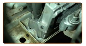
Tighten the upper fasteners of the engine mount. Use an 18 mm socket. Use a torque wrench. Tightening torque: 115 N·m.
