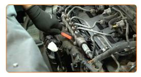
Unscrew the fasteners that connect the air intake hose to the intake manifold. Use a 13 mm socket. Use an 8 mm socket. Use a ratchet wrench. Use a U-joint socket extension.
