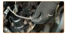
Attach the glow plugs power cable terminal and screw on the nut that secures it. Use an 8 mm socket. Use a ratchet wrench.
