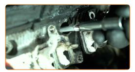
Tighten the glow plugs. Use a 10 mm glow plug socket. Use a torque wrench. Tightening torque: 13 N·m.
