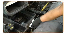
Plug the oil dipstick hole with a paper towel to prevent dirt from entering the system.
