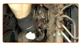
Plug the air intake hose with a paper towel to prevent dust and dirt from getting into the system.
