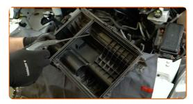
66 Install the air filter housing.
