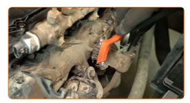
Unscrew the fasteners of the oil dipstick tube bracket. Use an 8 mm socket. Use a ratchet wrench.
