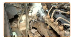
Unscrew the nut that secures the glow plugs power cable terminal. Use an 8 mm socket. Use a ratchet wrench.
