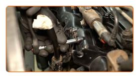
Treat the fuel pressure sensor connector. Use an electronic spray.
