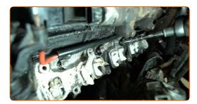
Clean the intake manifold mounting seat. Use a gasket scraper. Use an all-purpose cleaning spray.
