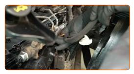
Attach the camshaft position sensor connector.
