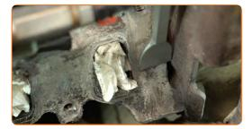
Remove the intake manifold gaskets.
