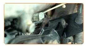
Treat the camshaft position sensor connector. Use an electronic spray.
