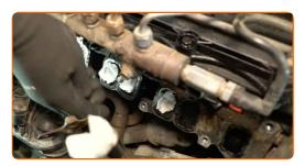
Unscrew the nuts that connect the power terminals to the glow plugs. Use a 7 mm socket. Use a ratchet wrench.
