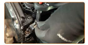
Detach the fuel pressure sensor connector.
