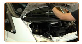
Use a fender protection cover to avoid damaging the paintwork and plastic parts of the car.
