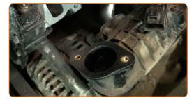
Install the intake manifold.
