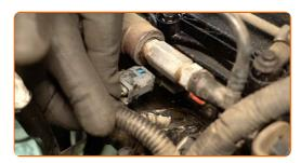
Detach the wiring harness fastener and move the harness aside. Use a clip removal tool.
