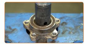
Clean the grease from the inner part of the bearing that remains on the hub, using a cloth.
