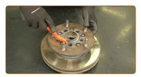
Unscrew the brake disc fasteners. Use a 13 mm socket. Use a ratchet wrench.
