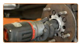
Remove the axle washer. Use a telescoping magnetic pick-up tool.
