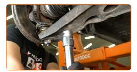
Tighten the wheel bearing fastening bolts. Use a T50 Torx bit. Use a torque wrench. Tightening torque: 53 N·m.
