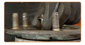
Detach the brake disc from the wheel hub.
