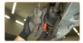
Unscrew the brake caliper bracket fasteners. Use an 18 mm socket. Use a tommy bar.
