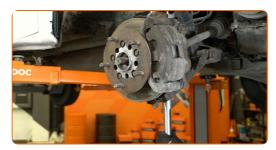
Detach the CV axle from the steering knuckle. Use a pin punch. Use a hammer.
