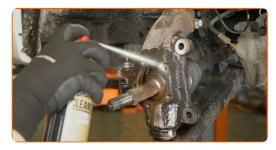
Clean the mounting seat of the brake caliper bracket. Use a wire brush. Use an all-purpose cleaning spray.
