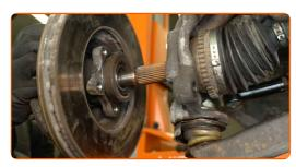
Clean the wheel bearing mounting seat. Use a wire brush. Use an all-purpose cleaning spray.
