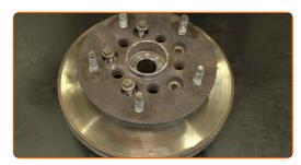
Screw in the brake disc fasteners. Use a 13 mm socket. Use a ratchet wrench.
