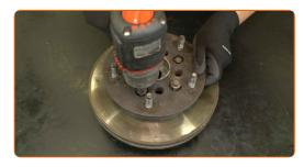
Treat the mounting surface on the wheel bearing. Use ceramic grease.
