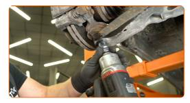
Support the steering knuckle. Use a transmission jack or one more vehicle jack.
