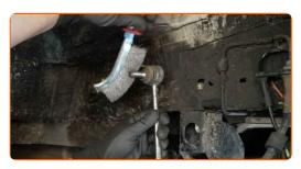
Clean the splines of the CV axle joint. Use a wire brush. Use an all-purpose cleaning spray.
