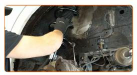
Screw on the strut mount fasteners. Do not tighten them.
