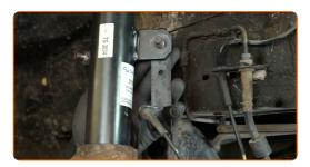
Tighten the fastener connecting the anti-roll bar link to the suspension strut. Use a 19 mm socket. Use a torque wrench. Tightening torque: 55 N·m.
