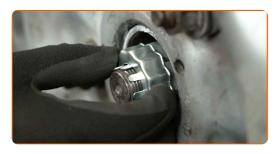
Install the cotter pin. Use a mounting lever.
