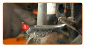
Unscrew the fastener of the ABS sensor cable bracket. Use an 18 mm socket. Use a ratchet wrench.
