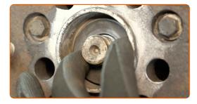
Screw on the axle nut. Use a 36 mm socket. Use a ratchet wrench.
