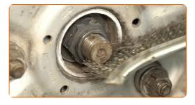
Loosen the axle nut. Use a 36 mm socket. Use a tommy bar.
