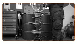
Remove the mount bearing and the bump stop.
