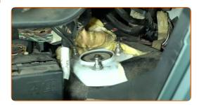
Clean the fasteners of the top strut mount. Use a wire brush. Use WD-40 spray.
