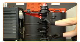
Remove the strut assembly from the spring compressor.
