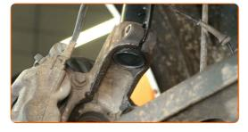
Install and screw in the fastening bolt.
