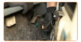
Unsnap the lock rod that connects the lock to the exterior door handle.
