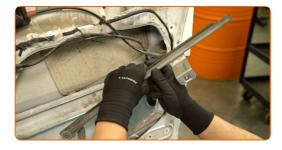
Unscrew the door lock fasteners. Use a T30 Torx bit. Use an electric or ratchet screwdriver.
