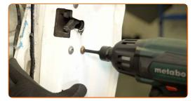
Remove the fastening screws.
