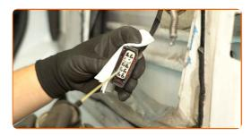
Attach the door latch cable to a new door lock.
