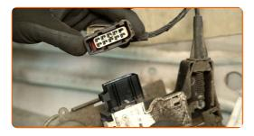
Detach the door latch cable from the lock.
