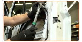
Snap into place the lock rod that connects the lock to the exterior door handle.
