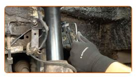
Clean the mounting seats of the anti-roll bar link on one side of the axle. Use a wire brush. Use an all-purpose cleaning spray.
