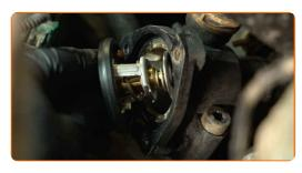
18 Install the thermostat housing cover.
