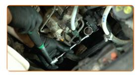
Remove the towel from the coolant hose and reattach it. Use hose clamp pliers.
