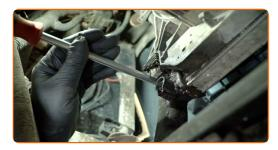
Loosen the coolant hose clamp. Use hose clamp pliers.
