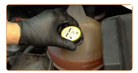
Run the engine for a few minutes. This should be done in order to remove residual air from the cooling system and to check that the components are operating correctly and there are no leaks.
