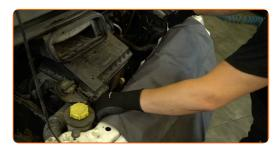
3 Unscrew the coolant reservoir cap.
