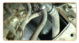
Unscrew the coolant drain plug. Use a slotted screwdriver.
