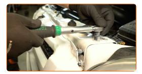
Install and screw in the upper fasteners of the radiator grille. Use a T30 Torx bit. Use a ratchet wrench.
