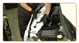
Install and screw in the fastening bolts of the upper radiator support cover.
