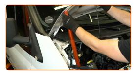
Attach the lower coolant hose. Use hose clamp pliers.
