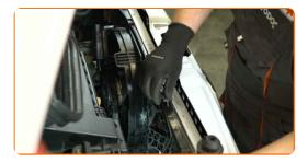
Remove the plug from the overflow hose and attach its connector to the radiator.
