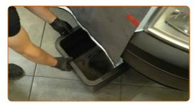
6 Unscrew the coolant drain plug. Use a slotted screwdriver.
