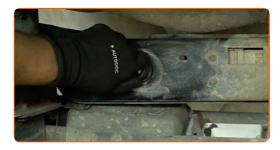
Remove the engine cooling fan shroud together with the fan from the radiator. Use a mounting lever.
