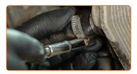
Screw in the coolant drain plug.
