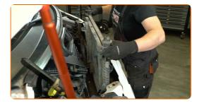
Remove the lower insulators of the radiator.
