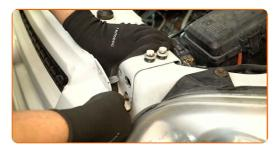
Tighten the fasteners of the upper radiator support cover. Use a 13 mm socket. Use a torque wrench. Tightening torque: 22 N·m.
