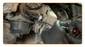
Detach the coolant hose from the oil cooler.
