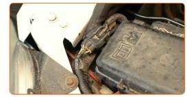
Attach the upper coolant hose. Use hose clamp pliers.
