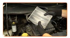
Close off the air duct using a clean towel and clean the inside of the cabin filter housing. Use a microfibre towel.
