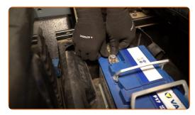
Screw in the negative battery terminal fastener. Use a 10 mm socket. Use a ratchet wrench.
