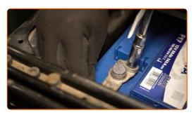
Connect the negative terminal to the battery.
