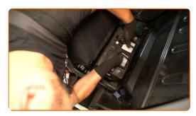
Clean the battery terminals. Use a battery terminal brush.
