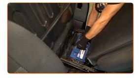
Connect the positive terminal to the battery.
