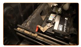
Remove the positive terminal from the battery.
