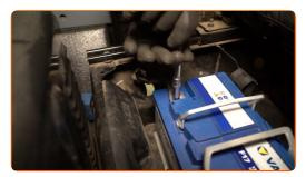
Reinstall the cover on the battery compartment.
