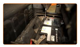
Remove the negative terminal from the battery.
