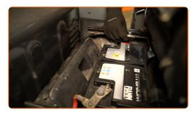
Unscrew the positive battery terminal fastener. Use a 10 mm socket. Use a ratchet wrench.
