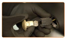
Treat the connector of the side indicator light. Use an electronic spray.
