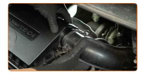
Snap the air intake hose clips into place.
