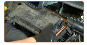
Plug the air intake hose with a microfibre towel to prevent dust and dirt from getting into the system.
