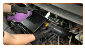
Connect the air intake hose to the air filter housing.
