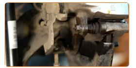
Unscrew the brake caliper fastening. Use a combination spanner #14. Use a combination spanner #17.
