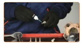
Clean the hub bearing mounting seat. Use a wire brush. Use WD-40 spray.
