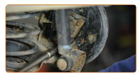
Remove the hub and the bearing together, since they are a sealed unit. Use a hammer.
