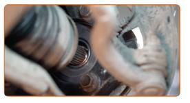
**42** Tighten the drive shaft nut. Use a drive socket #30. Use a tap wrench. Use a torque wrench. Tighten it to 216 Nm torque.
