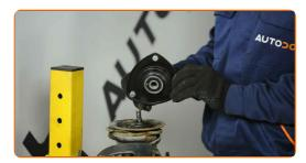
Tighten the shock strut piston rod nut. Use a drive socket #17. Use a torque wrench. Tighten it to 33 Nm torque.
