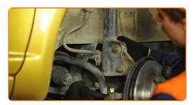
Tighten the brake hose fastening bracket to the shock strut. Use a drive socket #14. Use a ratchet wrench.
