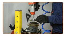
Remove the top strut mount. Use a flat screwdriver.
