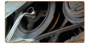
Place the V-ribbed belt on the alternator. Use a crowbar.
