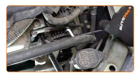
Tighten the alternator fasteners. Use a drive socket #12. Use a torque wrench. Tighten it to 15 Nm torque.
