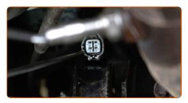
12 Attach the oxygen sensor connector.
