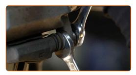
10 Remove the brake caliper.
