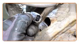
Clean the wheel hub fastener. Use a wire brush. Use WD-40 spray.
