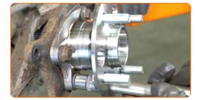
Treat the fasteners of the wheel hub bearing. Use copper grease.
