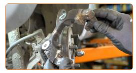
16 Remove the brake disc.
