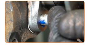
Tighten the wheel hub bearing fasteners. Use a drive socket #14. Use a torque wrench. Tighten it to 90 nm torque.
