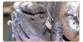
Remove the dust boot caps of the brake caliper guide pins. Use a crowbar.
