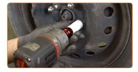
Lower the car and working in a cross order, tighten the wheel bolts. Use wheel impact socket #21. Use a torque wrench. Tighten it to 103 Nm torque.
