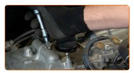
Screw new spark plugs and tighten them. Use the spark plug socket #16. Use a torque wrench. Tighten it to 20 nm torque.
