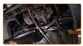
Unscrew the drain plug. Use a drive socket #15. Use a ratchet wrench.
