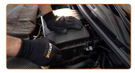
Install the fastening clamps of the air filter breather pipe and the air filter inlet pipe. Use hose clamp pliers with retainer.
