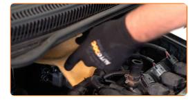
Reinstall the air filter cover. Fasten it.
