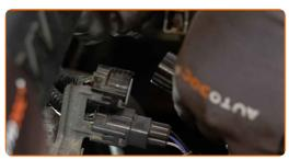
Unfasten the clamp to release the oxygen sensor wiring harness. Use a flat screwdriver.
