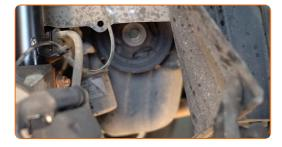
Clean the tensioner pulley of the V-ribbed belt. Use WD-40 spray.
