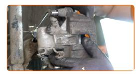
Tighten the brake caliper fasteners. Use HEX No.H7. Use a torque wrench. Tighten it to 34 nm torque.
