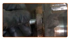
Tighten the brake caliper bracket fasteners. Use a drive socket #14. Use a torque wrench. Tighten it to 57 Nm torque.
