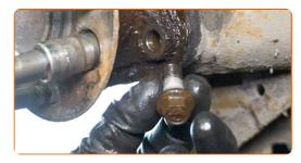
Remove the hub and the bearing together, since they are made as an assembly. Use a crowbar. Use a hammer.
