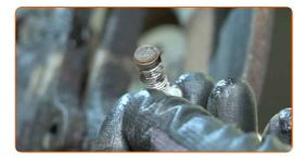
Remove the caliper bracket.
