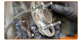
Clean the hub bearing mounting seat. Use a wire brush. Use all-purpose cleaning spray.
