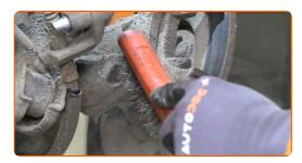
Unscrew the brake caliper bracket fasteners. Use a drive socket #14. Use a ratchet wrench.
