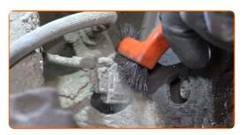
Detach the ABS sensor connector. Use a flat screwdriver.
