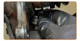
Screw in the fastener that connects the shock strut to the steering knuckle. Use a combination spanner #19. Use a drive socket #19. Use a ratchet wrench.
