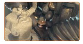
Tighten the brake caliper bracket fasteners. Use a drive socket #17. Use a torque wrench. Tighten it to 107 nm torque.
