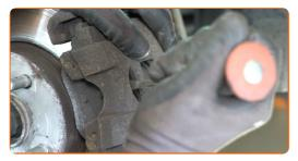
Remove the brake caliper. Use a crowbar.
