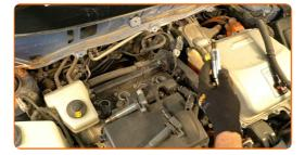
Apply a thin layer of a special high temperature anti-seize lubricant to the threads of the new spark plugs.
