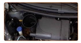
Pour oil into the engine through the filler. Required amount of oil: 3.6 L.
