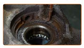
Remove the wheel hub bearing retaining ring. Use circlip pliers.
