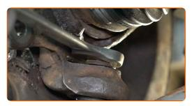
Tighten the fastener connecting the ball joint to the steering knuckle. Use a combination spanner #19. Use a torque wrench. Tighten it to 65 Nm torque.
