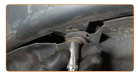
Remove the side bumper retainer clips. Use a Phillips screwdriver. Use a clip removal tool.
