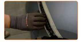
Carefully release the bumper from the fasteners.
