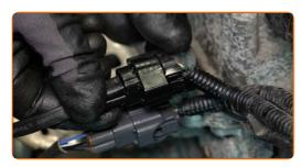
Fasten the oxygen sensor wiring with the clamp.
