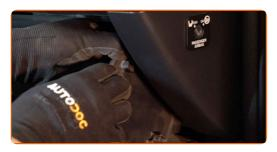
A Remove the cabin filter housing cover.
