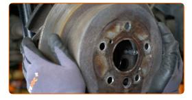
Remove the left brake shoe spring of the parking brake. Use long nose pliers. Use a crowbar.
