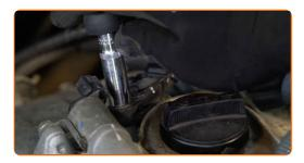
7 Take out the ignition coils from the spark plug wells.
