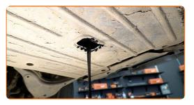
Replacement: engine oil and filter – TOYOTA Tundra Pickup (\_K3\_, \_K4\_). Tip:
