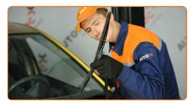
Remove the blade from the wiper arm.
