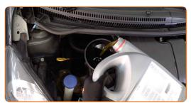
Replacement: engine oil and filter – TOYOTA Tercel I Hatchback (L10).
