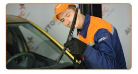
Remove the blade from the wiper arm.
