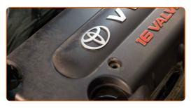
Screw in the engine cover fasteners. Use a drive socket #10. Use a ratchet wrench.
