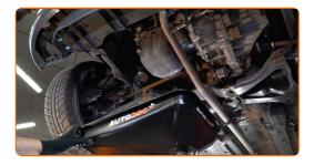
Unscrew the oil filter. Use the 76/14-F socket. 9
