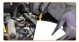
Reinstall the wiring harness bracket.
