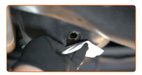
Screw in the new drainage plug and tighten it. Use a combination spanner #14. Use a torque wrench. Tighten it to 25 Nm torque.
