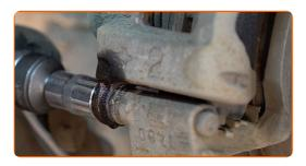
10 Remove the brake caliper.
