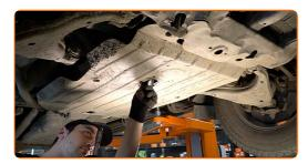
Screw in the new oil drain plug. Use a drive socket #17. Use a ratchet wrench.
