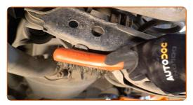
Unscrew the fastener connecting the stabilizer link to the control arm. Use a drive socket #17.
