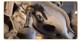
Unscrew the fasteners connecting the stabiliser link to the stabiliser bar. Use a drive socket #17. Use a ratchet wrench.
