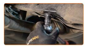
Tighten the fastener connecting the stabilizer link to the stabilizer bar. Use a drive socket #17. Use a torque wrench. Tighten it to 74 Nm torque.
