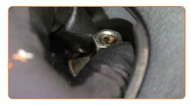
Remove the elements of the shock absorber upper mount.
